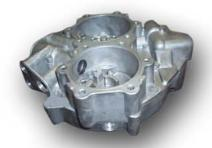
In the die-casting procedure the aluminium- resp. zamak-melt is injected under high pressure and high velocity through a piston into a a one- or more-part permanent form. The die casting procedure offers a very good technical and economic solution for the utilization of aluminium or zamak-parts with complicated forms.
